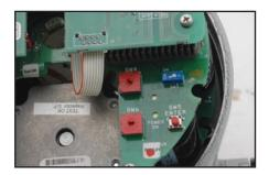
Easily accessible control panel helps allow setting of torque, speed, and position quickly and simply. All settings are done from this control panel.
